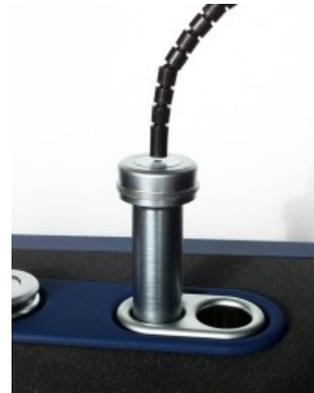
3. Position the reference microphone (1) pointing straight down from above and centered 1-2 millimeters above the coupler measurement microphone (3).
