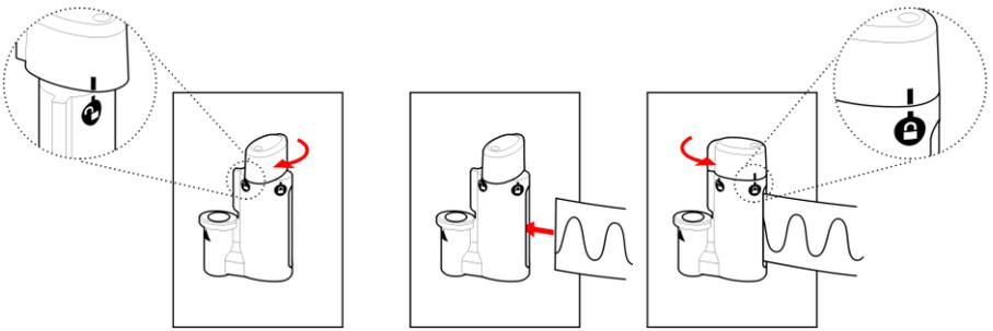
Twist the top end of the Belt Lock clockwise to open the catch. The white mark on the top should match the open lock symbol on the catch.
