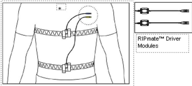
7. Plug the thorax module output into the appropriate bipolar input of your polygraph. The red touch-proof plugs into (+) input, and the black plugs into (-) input.
